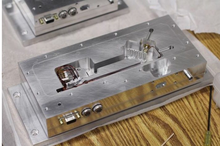
Abbildung 0.1: Picture of an ECDL. The missing grating and biprism pair were added later.
